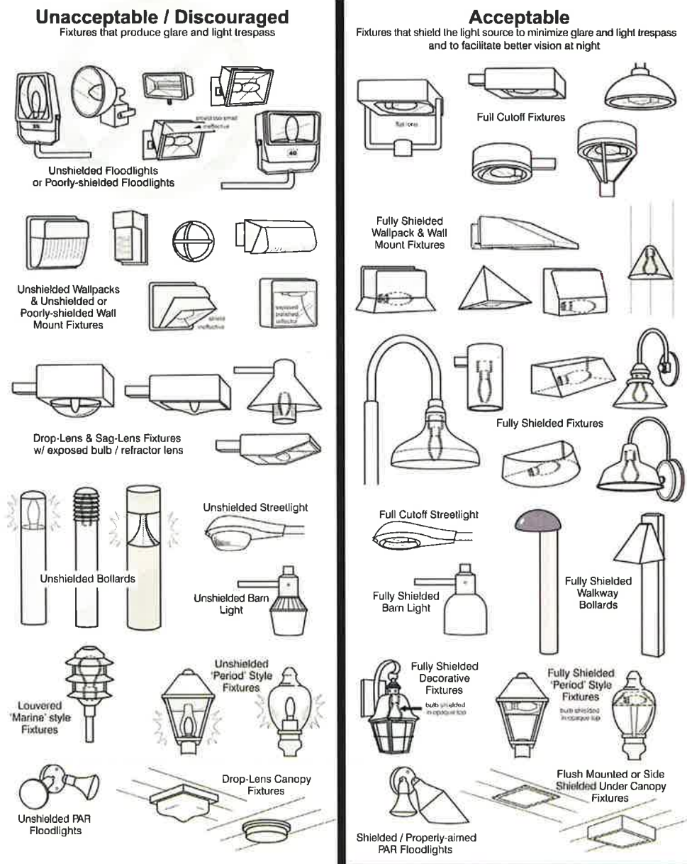
Figure 5.9 - Acceptable Light Fixture Types (From darksky.org)
